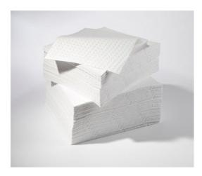
Our range of **Spilchoice Medium Weight Oil & Fuel Pads** are an ultrasonically bonded hydrophobic pad that delivers an absorbency rate of 1 liter per pad and are designed to selectively absorb **oil based liquids** such as fuels, lubricants and other hydrocarbon based products. Our oil absorbents are hydrophobic, meaning that they can be used for the selective recovery of oil from water.
