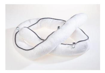
The **Absorbent Boom (3000mm x 200mm)** has been developed for the containment and **absorption of oil spills and debris** in rivers and harbors. The boom has a **polypropylene inner** and can absorb **40 liters of oil** and diesel spills and can cover large areas by overlapping the booms with the fitted clips and rings.
