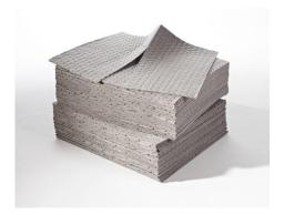
Our range of **Light Weight pads** are a melt blown, ultrasonically bonded with spaunbond, highly versatile absorbent that can be used inside working environments to absorb most oil and water based liquids including paints, solvents, coolants and mild chemicals.
