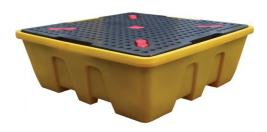
The **Stackable Double IBC Spill Pallet** is a sturdy and durable secondary containment system designed for the storage of two standard 1000 litre IBC. The IBC can be positioned on the integral load bearing columns for full support and is designed to be stacked in 9 making it highly efficient.
